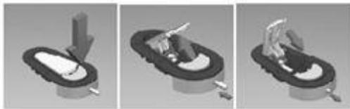
**Before starting to install your AeroCatch, Check which version of shear pin is fitted. If you have a stainless steel uncoated shear pin (see Fig 1) lubricate the inside linkage and shear pin with a light spray oil wiping away any excess. If you have a stainless steel shear pin with a PTFE coating (see Fig 2) additional lubrication is NOT NECESSARY as the PTFE Coating provides all the lubrication needed to operate the AeroCatch.**
